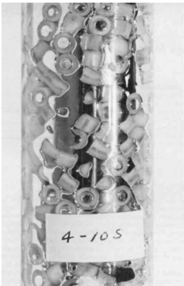
Fig. 8. Countercurrent flow of mercury and water through a 2.54-cm (1-in)-diam column packed with 0.476 cm (3/16 in) Raschig rings. Superficial water and mercury velocities were 0.0787 and 1.57 cm/s, respectively.
